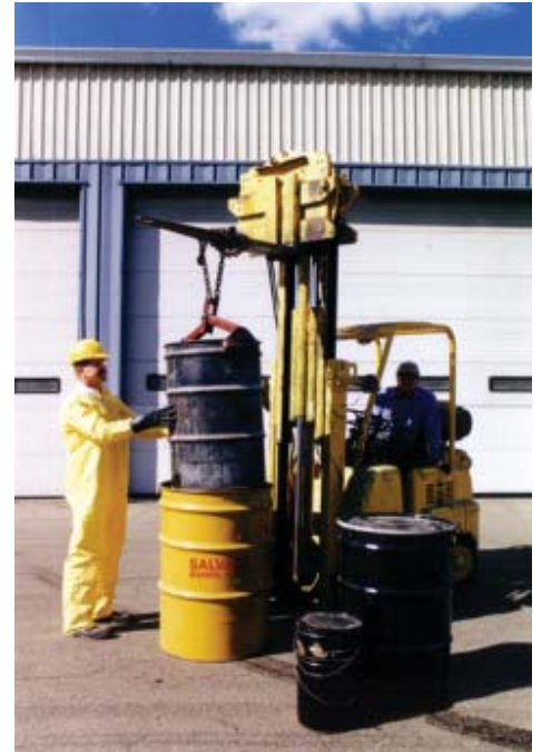
Lowering a loaded drum into an overpack for transport at Valley City Environmental Services, Inc.
