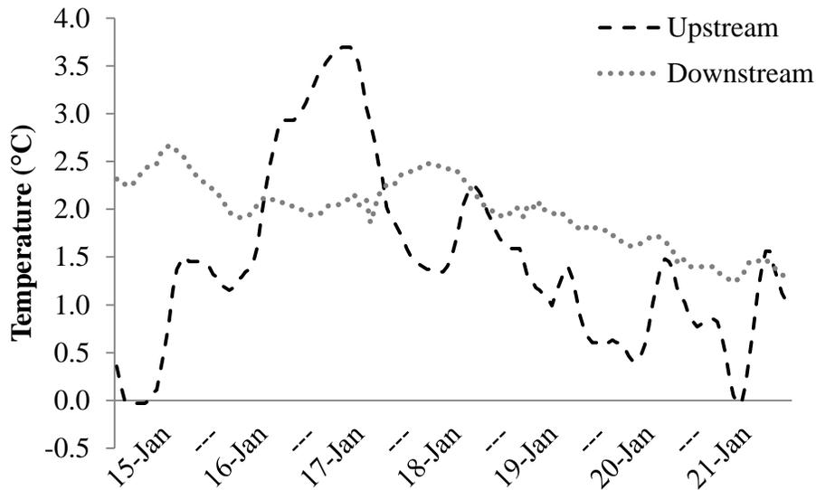
**Figure 4a.** Hourly water temperature during the week of 15 January 2012. Water temperature was recorded each hour using HOBO Pendant Temperature Loggers (Model: UA-001-08; Onset Computer Corporation) at an upstream site (near Grasshopper Ranch Upper (A)) and a downstream site (near Garfield Road Lower (D)).
