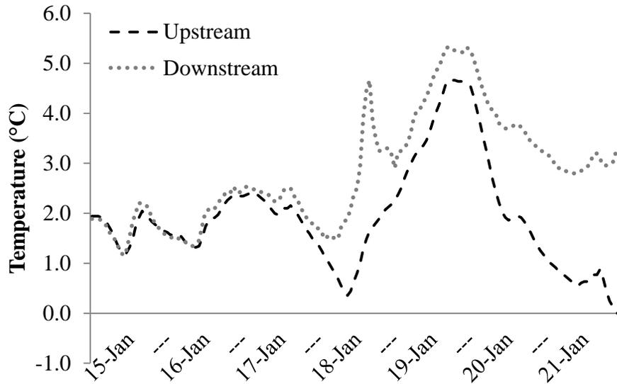
**Figure 4b.** Hourly water temperature during the week of 15 January 2013. Water temperature was recorded each hour using HOBO Pendant Temperature Loggers (Model: UA-001-08; Onset Computer Corporation) at an upstream site (near Grasshopper Ranch Upper (A)) and a downstream site (near Garfield Road Lower (D)).
