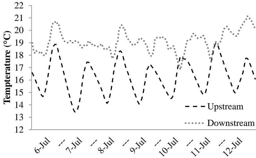
**Figure 3a.** Hourly water temperature during the week of 06 July 2011. Water temperature was recorded each hour using HOBO Pendant Temperature Loggers (Model: UA-001-08; Onset Computer Corporation) at an upstream site (near Grasshopper Ranch Upper (A)) and a downstream site (near Garfield Road Lower (D)).
