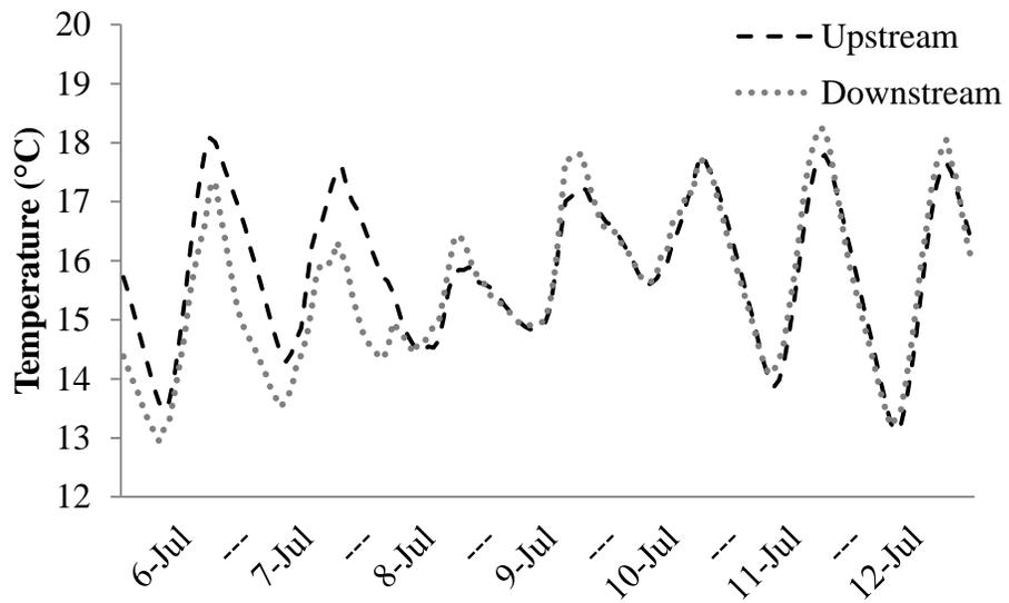
**Figure 3b.** Hourly water temperature during the week of 06 July 2013. Water temperature was recorded each hour using HOBO Pendant Temperature Loggers (Model: UA-001-08; Onset Computer Corporation) at an upstream site (near Grasshopper Ranch Upper (A)) and a downstream site (near Garfield Road Lower (D)).
